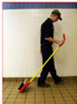
**To transport:** simply pull the pole past the rest position on to its wheels and roll away.
