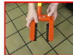
To adjust brush size, loosen the wing nut and slide brush to desired position then tighten nut.
